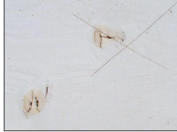
Fig. 2.7: Discoloration of the coating system due to wood substances in the knot area
