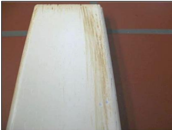
Fig. 2.5: Discoloration of the coating system due to wood substances
