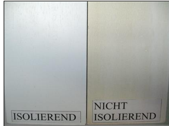
Fig. 2.6: Comparison of the insulating effect of a coating system with and without insulating filler
