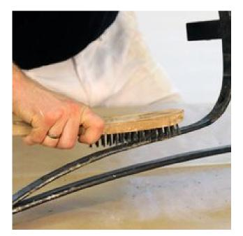
Step 3: Grinding and cleaning the metal
