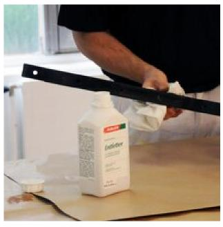
Use grinding fleece for grinding and ADLER Entfetter over the metallic surfaces for thorough cleaning. After allowing it to act for 5-10 min., you can rewash with clear water and allow everything to dry.
