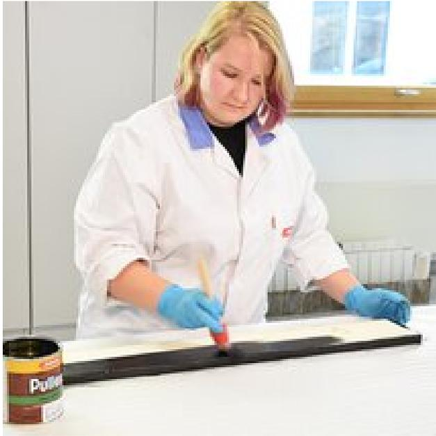
You can then paint the large area in full. Allow the board to dry off for 4 to 6 hours. After this time the board is not yet dried through.
