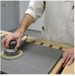
The filled, dry substrate should then be sanded directly with grit 240 before painting.
