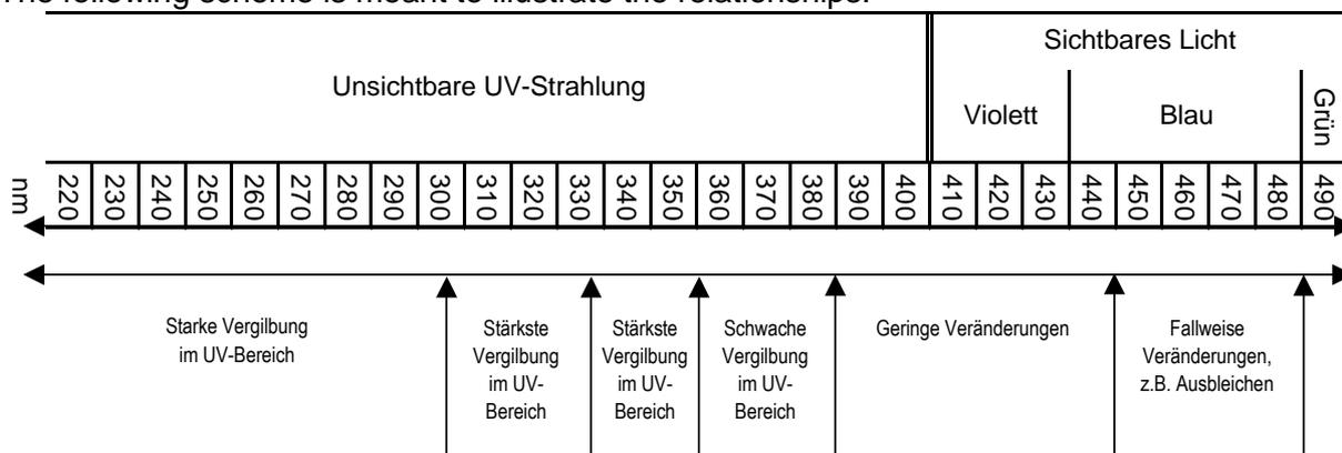
Bleaching occurs as a colour-related change in wood resulting from decomposition of the wood dyestuffs, yellowish (yellowing) or red discoloration as well as darkening is caused by the decomposition of wood extractives and formation of new dyestuffs at the same time.
